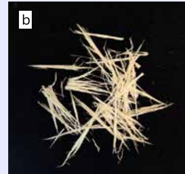
Figure 2: Results from Drafting. (a) Initial Sample with increased water content of 400% after passed through the drawing frame along the fiber axis (b) Initial Sample with increased water content of 400% after passed through the drawing frame at 45° orientation
