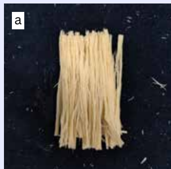
Figure 2: Results from Drafting. (a) Initial Sample with increased water content of 400% after passed through the drawing frame along the fiber axis (b) Initial Sample with increased water content of 400% after passed through the drawing frame at 45° orientation
